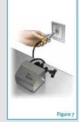
Ensure the Flow Regulator is connected to a compressed air or Nitrogen source (Figure 7).
