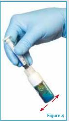
Gently shake vial/syringe assembly until powder is completely dissolved. The solution will turn blue (Figure 4).
